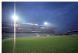
Conventional CCD Sensor (vertical smear)
